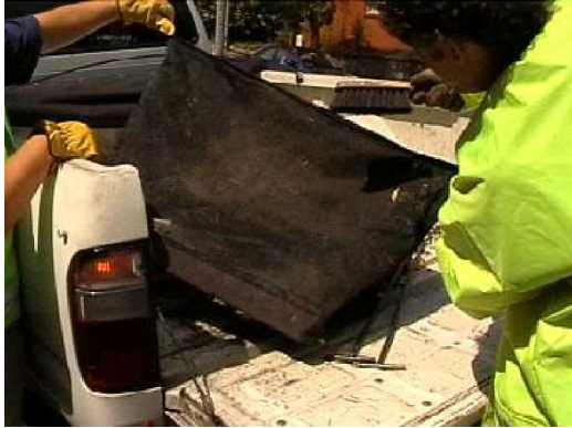
Plate 31 Slightly clogged filter bag, indicated by the brown stain on in the centre of the bag
